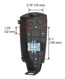
3. Attach the bracket using fasteners that are appropriate for the type of wall material, drilling pilot holes if necessary. Use the supplied screws only if mounting the bracket directly to a wooden stud. If mounting to another type of wall (hollow, masonry, etc.), use fasteners that are long enough to securely anchor the Wall Connector and can hold at least 80 lb (36 kg).
