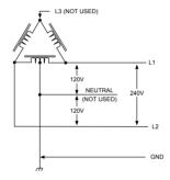
(L3 in the illustration) of the delta is 208V, with respect to neutral, and is sometimes. referred to as a "stinger." Do not use this third line.
