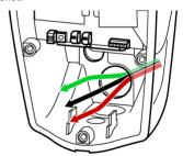
3. Strip the service wires going to the terminal block on the top entry bracket 3/4" (18 mm). Ferrules are recommended.
