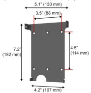
For U.S.A. installations, position the bracket so that the Wall Connector is located at a maximum of 60" (150 cm) from floor level. The minimum height is 18" (45 cm) if mounting indoors.
