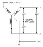
↑ Caution: The unused leg (L3 in the illustration) must remain open. Do not connect to a neutral bar, or to earth around.
