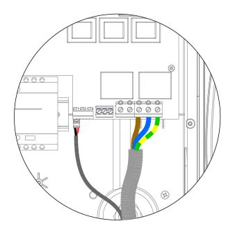
For single phase installations where 1 or 2 external / hardwiring an external CT please follow the above additional CT's are required, please follow the above diagram to connect the CT's using the extra 2 CT terminals in the same way if required. Positive (+) = Red Negative (-) Black
