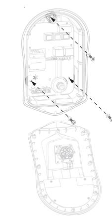
Using the fixing kit provided secure unit to the wall ensuring the grommets are used to maintain its IP integrity (Note: if using the rear cable entry remember to insert the mains cable before mounting to the wall!) 6
