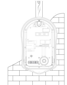
Using zoppi template mark mounting holes. Use top and 2 bottom holes left/right for brick use 2 vertical holes if mounting to a stud wall or joist.
