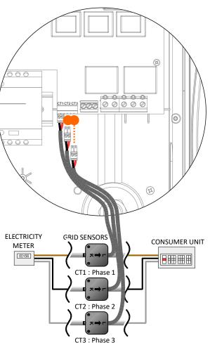
**SINGLE PHASE:** A CT clamp must be placed around the live meter tail as shown above with the arrow pointing towards the consumer unit.
