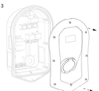
Remove all 8 screws from the enclosure and carefully lift away.
