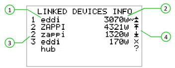
This screen lists all the linked devices (1) and the priority setting for each device (3) The current device is shown in CAPITAL letters. To the right of each device is the real-time output power level (2) The right side of the screen has symbols to show the status of each device (4) Refer to the table below for the meaning each symbol.
