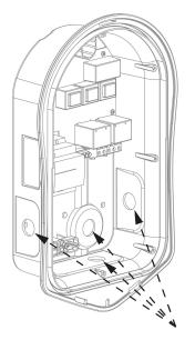
There are 4 possible cable entry positions, carefully decide which one you are going to use from the above image. You will need an IP65 or above rated cable gland. Carefully drill hole into unit to match the size of your cable gland. Attach cable gland ensuring IP rating is met.
